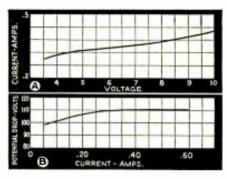
A—Average characteristic curve of the gaseous type of regulator tube. The WL-706 is considered typical of its class.
